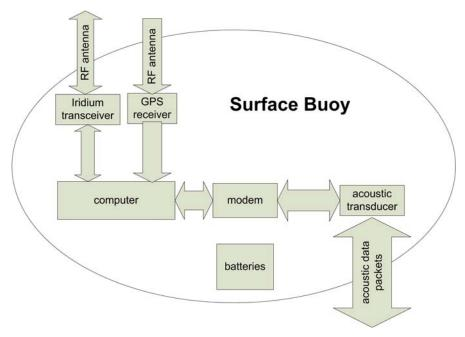
Figure 5: Block diagram of DART II surface buoy.
