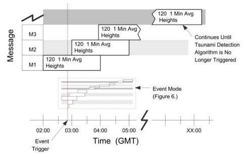
Figure 7: Timing diagram during Extended-Reporting Mode
