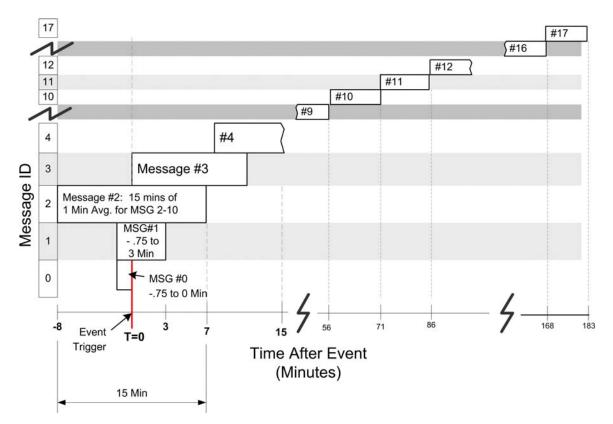
Figure 6: Timing diagram showing messages during Event Mode.
